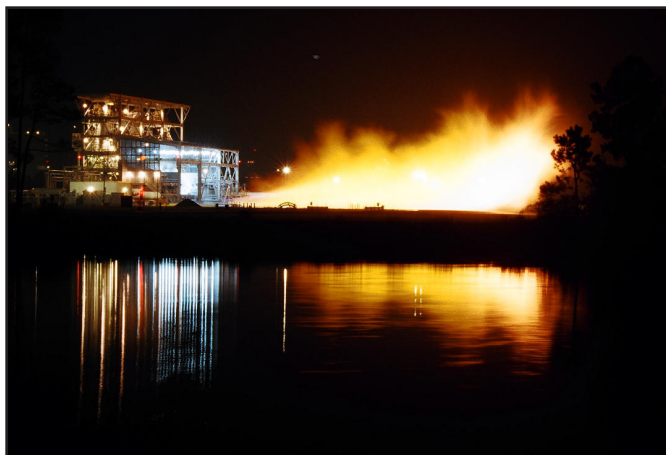
A test of the Integrated Powerhead Demonstration liquid hydrogen turbopump is conducted on the E-1 Test Stand at SSC's E Complex.
